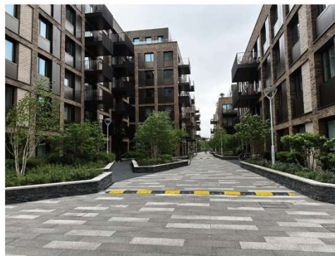
Avoid Traffic calming should be integrated from the outset in new streets. Avoid retrofitting products in clashing materials/colours.
